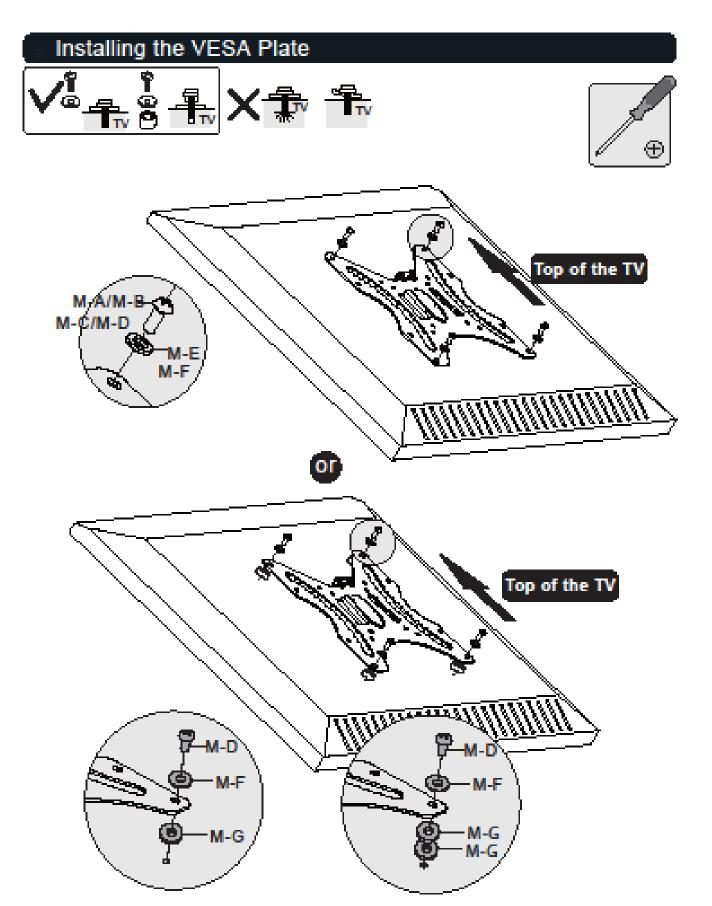
Note: Choose the appropriate screws, washers and spacers (if necessary) according to the type of screen. Screw the VESA plate onto the TV.
