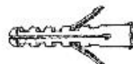
(6) Concrete Anchors - f
