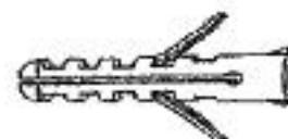
(6) Concrete Anchors - f
